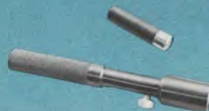
The URT-33 personnel locator beacon (above left) should be broadcasting your position as you float down. The RT-10 (above right) is currently being replaced by either the PRC-90 (dual channel) or the URC-64 (multi-channel).
