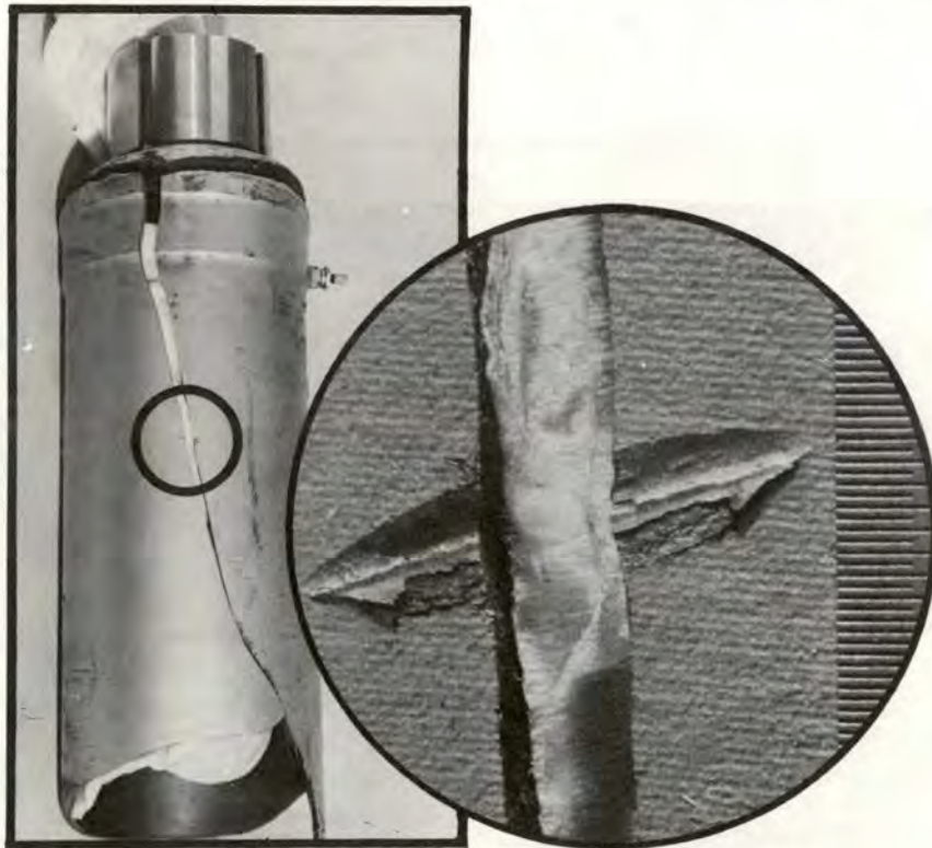
Fractured cylinder that finally failed from corrosion under small nick shown in lower right photo. Tiny nick, just .6" long and .015" deep, escaped observation.
