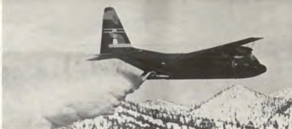
Modular airborne fire fighting system allows dispersal of fire retardant evenly over a 1200'x150' area. System can be installed in C-130 in few hours.
