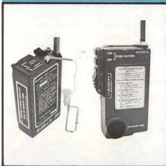
The URT-33 personnel locator beacon (above left) should be broadcasting your position as you float down. The RT-10 (above right) is currently being replaced by either the PRC-90 (dual channel) or the URC-64 (multi-channel).
